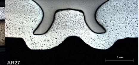
7075 sheet – Die Preheating 5-s at 365°C
