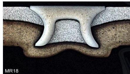
Al to Mg – Die Preheating 2-s at 360°C
