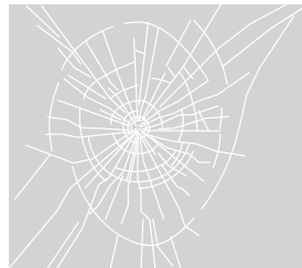
< Broken Laminated Glass >
