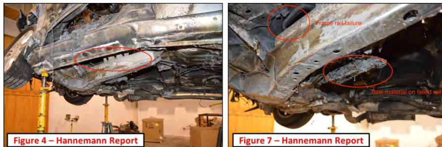
Figure 12 – Lower Frame Rail Deformation (Reproduced from Mr. Hannemann's Report)
