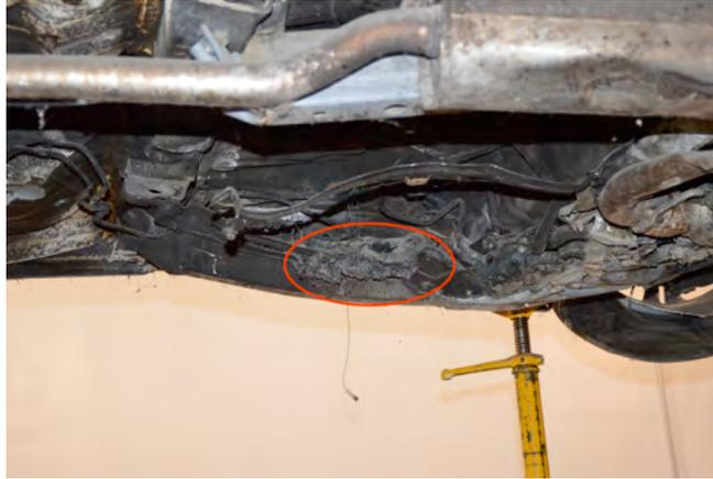
Figure 6 – Fuel tank material on failed structure
