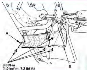
5. Except LX (A/T model): Remove the fuel tank cover (A).
