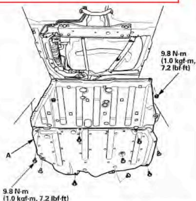
7. Remove the front floor cross beam (A), and the tank mount bracket (B).
