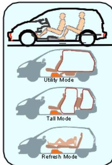
Figure 10 – Honda Fit fuel tank location and seating modes
