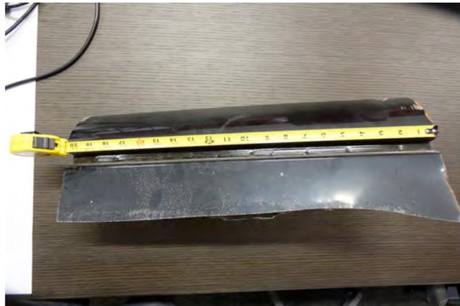
Figure 4 – Original Honda spot welding
