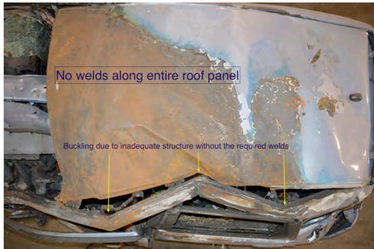
Figure 3 – Defectively repaired Honda Fit roof
