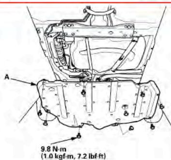
6. LX (A/T model): Remove the floor under cover assembly (A).
