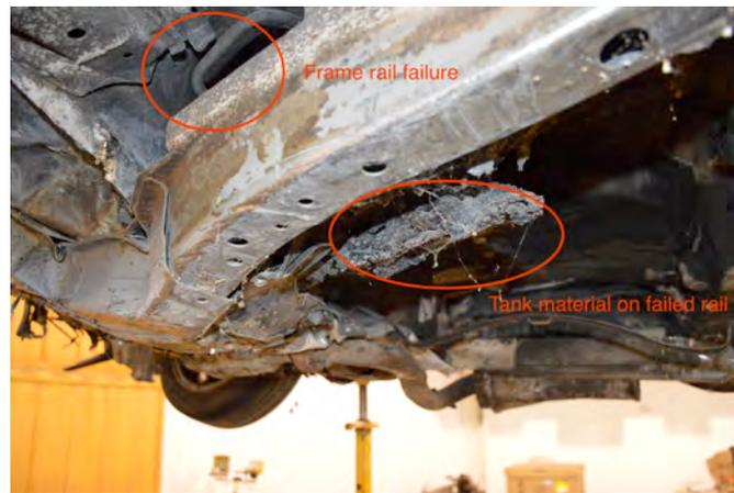
Figure 7 – Fuel tank material adjacent to failed structure
