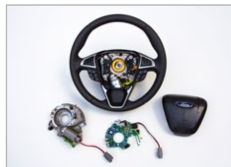
Adaptive Steering changes the ratio between the driver's input at the steering wheel and the amount the front wheels move.
