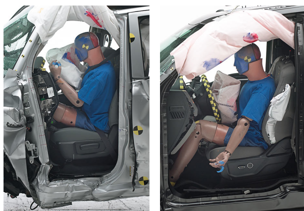
Extensive intrusion into the occupant compartment of the Ram 1500 Quad Cab (left) resulted in a poor rating for structure. In contrast, survival space for the dummy held up well in the Ford F-150 SuperCab (right), earning the pickup a good small overlap rating.
