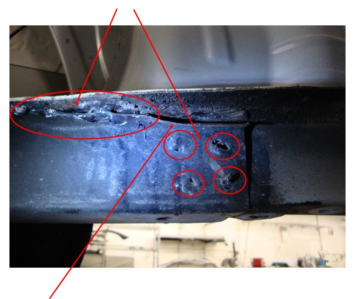
Gap between frame and floor due to remaining damage
