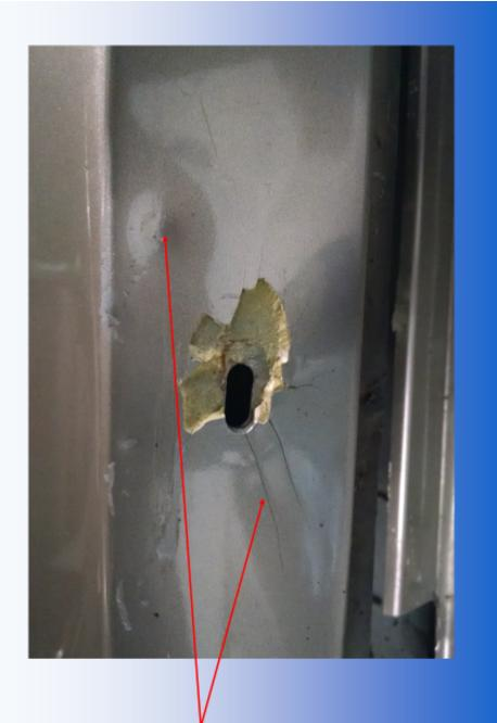
Viewed more closely, the rocker panel is noticeably cracked, bent, and dented. This panel should be smooth and straight with no bends or contours. Poor and incomplete welds lacking fusion. Note holes in the "welds," rust, and poor workmanship. THIS IS A SAFETY ISSUE.
