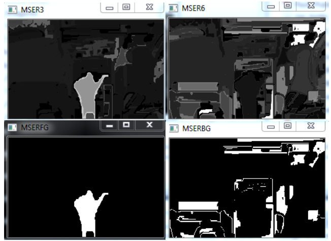
Figure 4: Combination of MSER and EBM modules. Top Left: Probability of Foreground regions, Top-Right: Probability of Background regions. Bottom row: thresholded probability images.
