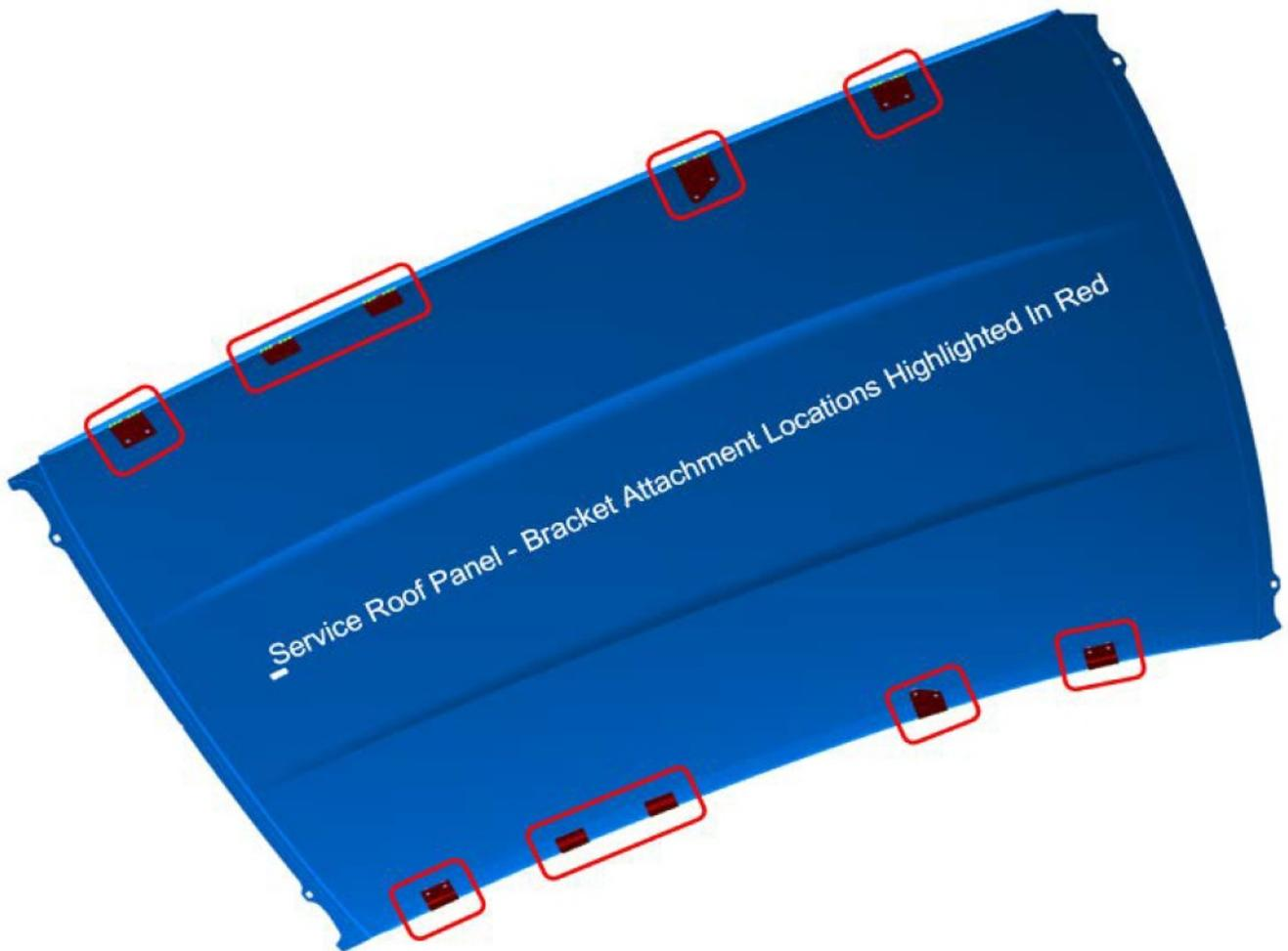
Service Replacement Roof Panel (Underside View)
