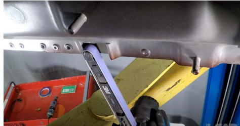
The use of different tools can help accommodate repairs over different types of contours and angles. Staying on the raised portion of the inner rocker panels allows the repairer to avoid the adhesive layer in the pinch-weld area.
